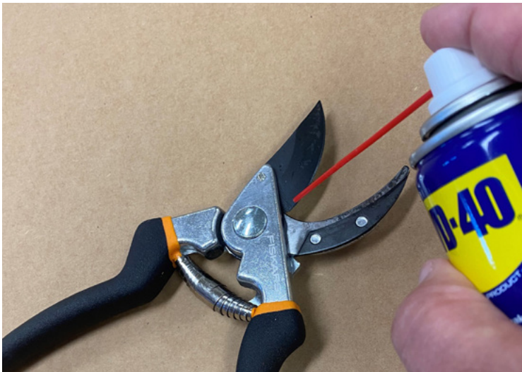
Add a light oil to cutting tools and wipe off excess after they have been sanitized.
